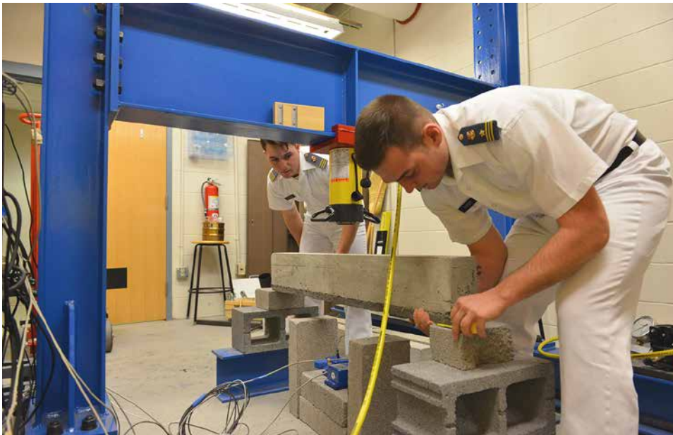
Devon Zappolo '18 and Jon Kaiser '18 prepare to test a concrete beam in a civil and environmental engineering lab.—VMI Photo by Mary Price.
