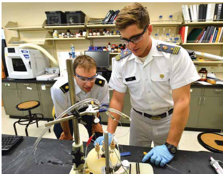
Maj. Dan Harrison '05 and Jake Hyde '17 set up a specially designed, air-free, electrochemical cell containing one of Hyde's iron compounds. – VMI Photo by Kelly Nye.
