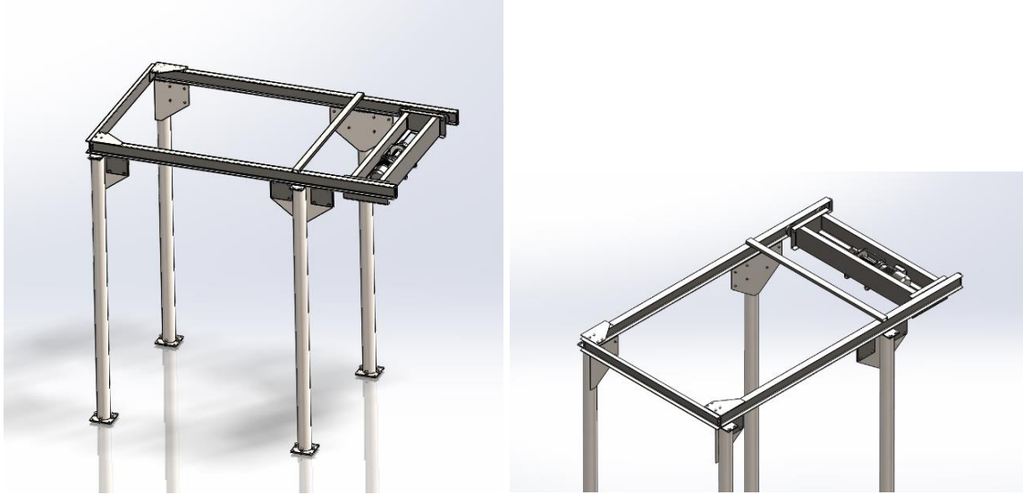
Figure 2: Double Track Gantry Design
